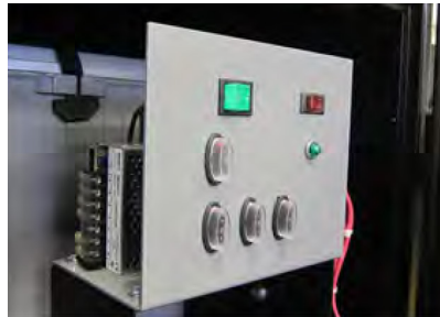
Control panel; Standard control panel can accommodate up to 4 individual 16 volts or 6 individual 12 volts
